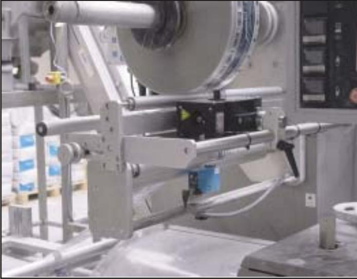
A candy manufacturer uses a Klockner-Hansel horizontal flow wrapper to individually pack large gum balls in a colored plastic film. The Hot Quick Coder is used to apply 3 lines of 2.5mm code to the film including product code, manufacturing date and expiration date.
