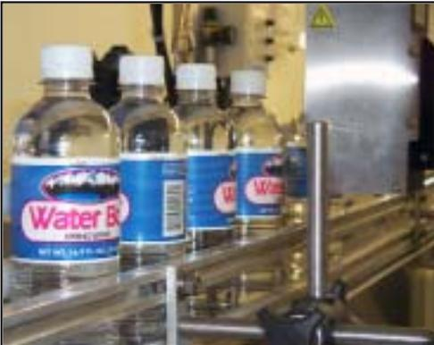
The date codes in this application are applied horizontally on the top edge of the labels on some of the production and directly on the crown of the bottles during production of unlabeled products. The codes applied by the Hot Quick Coder dry instantly even when the surface of the bottle is slightly wet.
