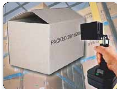
Hand-coding cartons on pallets with hand-held pack
