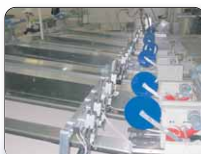
Printing multiple egg carton lines with single controller
