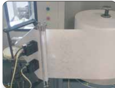
Printing dual-line text in 2 different colour on coil mattress sheath
