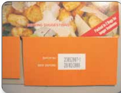
Printing use-by & batch codes on carton end-flaps
