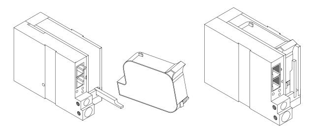
NOTE: WHEN A NEW CARTRIDGE IS INSTALLED, BOTH THE RED AND GREEN LIGHT WILL FLASH TWICE INDICATING A CORRECT INSTALLATION. THE USER MUST REMEMBER TO RESET THE INK LEVEL UNDER THE F4 FUNCTION KEY.
