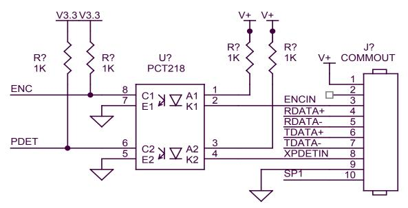
Each input requires the capability of sinking 12ma to ground as depicted in the above circuit. Connection to the optional control port requires an RJ50 connector.
