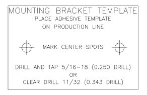
Locate the supplied mounting template and affix in a convenient location on the production line. Spot and drill both mounting holes for a 5/16" bolt. NOTE: the user may also thread the side of the conveyer using a 5/16" tap.
