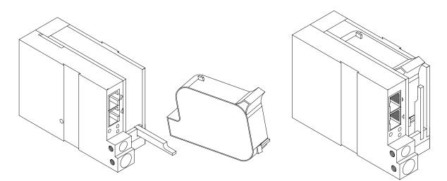
NOTE: WHEN A NEW CARTRIDGE IS INSTALLED, BOTH THE RED AND GREEN LIGHT WILL FLASH TWICE INDICATING A CORRECT INSTALLATION. THE USER MUST REMEMBER TO RESET THE INK LEVEL UNDER THE F4 FUNCTION KEY MENU.
