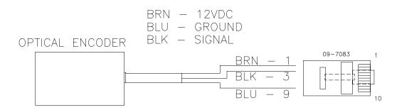
The above pictorial is an example of the connections for an external encoder.
