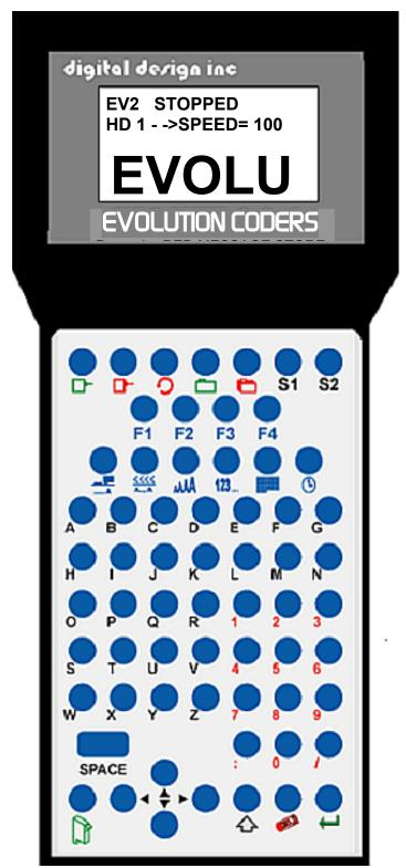
The keypad on the print station, pictured here, contains 64 keys. The LCD will display various messages to assist in programming on the upper half of the display. The lower half of the display will show up to two lines of the entered print message.
