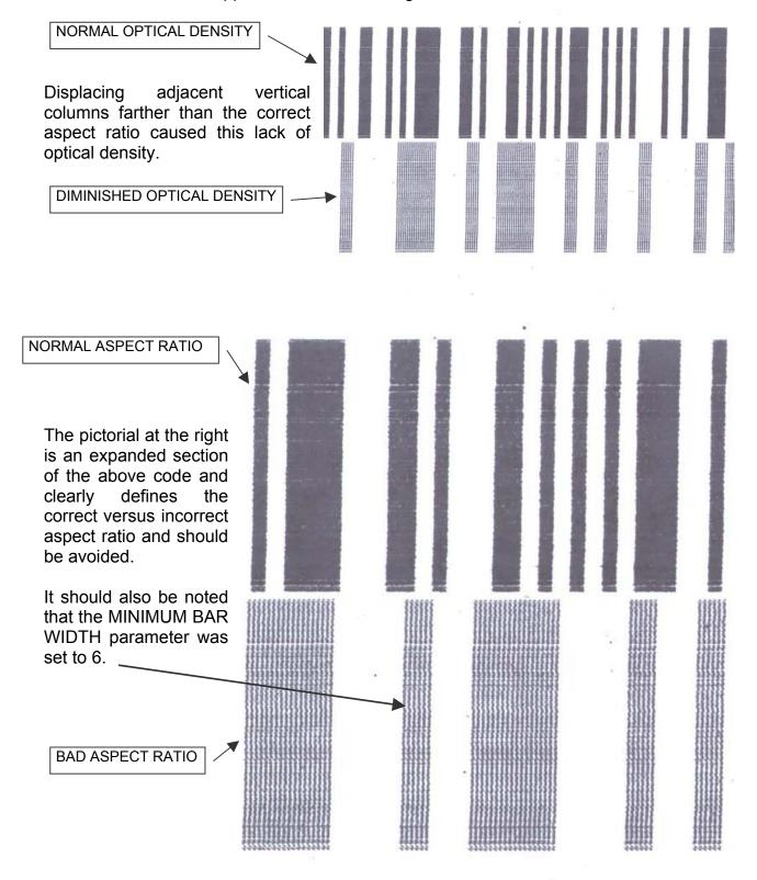
Below is a scanned image of a typical application where there was an acceleration and deceleration component in the line movement. Notice how the bars grew from left to right then began to compress towards the normal at the right. Also apparent is the change in the optical density of the pattern. This was a totally unreadable code.
