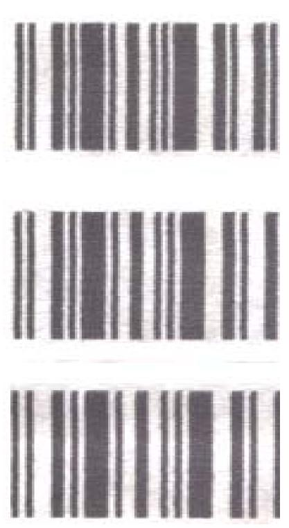
Bar growth will also lead to a less dense dark bar due to the fact the printed vertical columns will print further apart then previous dark bars. This may also be seen when not using an encoder and the line speed of the printer is set slower than the actual line speed of the production line.
