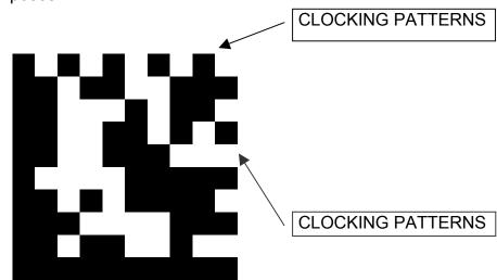
Data matrix codes are more tolerable to stretch and skew by the nature of their imbedded clocking patterns defining both columns and rows.
