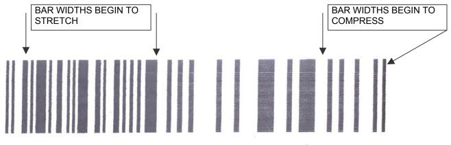
Finally, the image as it should look. This code was produced on white corrugated at 100ft/min and produced a verifiable class "A" with a decodability of 70%. The average bar growth from the reference standard was 0.03%.
