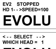
The hand held controller can program up to 32 print carriages on an RS485 data link. The factory default sets each print carriage to ADDRESS 1. Selection of another print head other than ADDRESS 1, press
