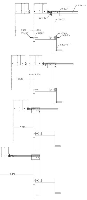
Vertical height adjustment for the EVOLUTION II print head is accomplished by loosening the included hand knob 5993K41.
